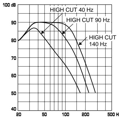
The figures below show the optimum adjustment of each control and the frequency characteristics when this subwoofer is combined with a typical main speaker system.
